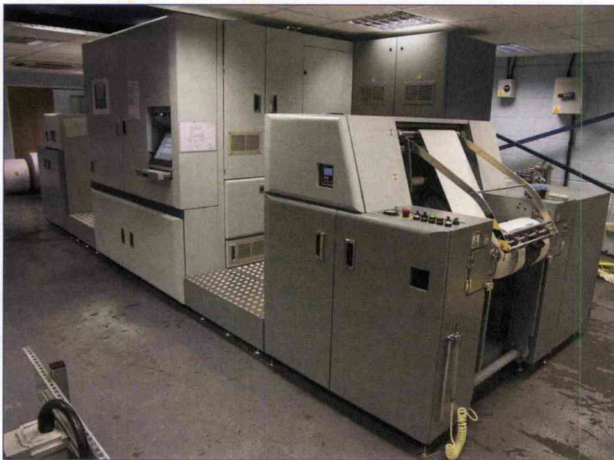
The JetStream 1000 runs roll to roll, seen with the delivery end nearest the camera.
