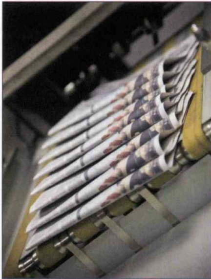
Newspapers are delivered off the Hunkeler nearline sheeting, collection and folding line.
